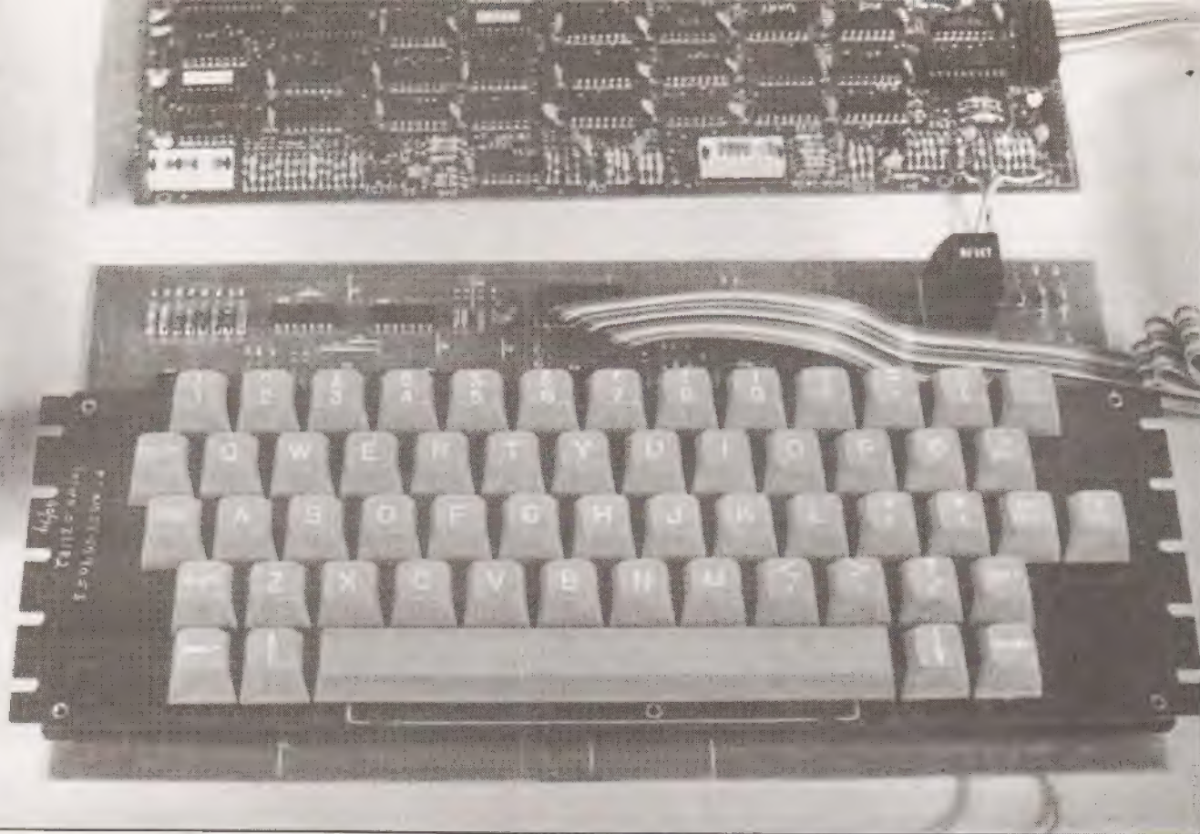
The new extended keyboard with full cursor control, RESET is still in a bad position though.
